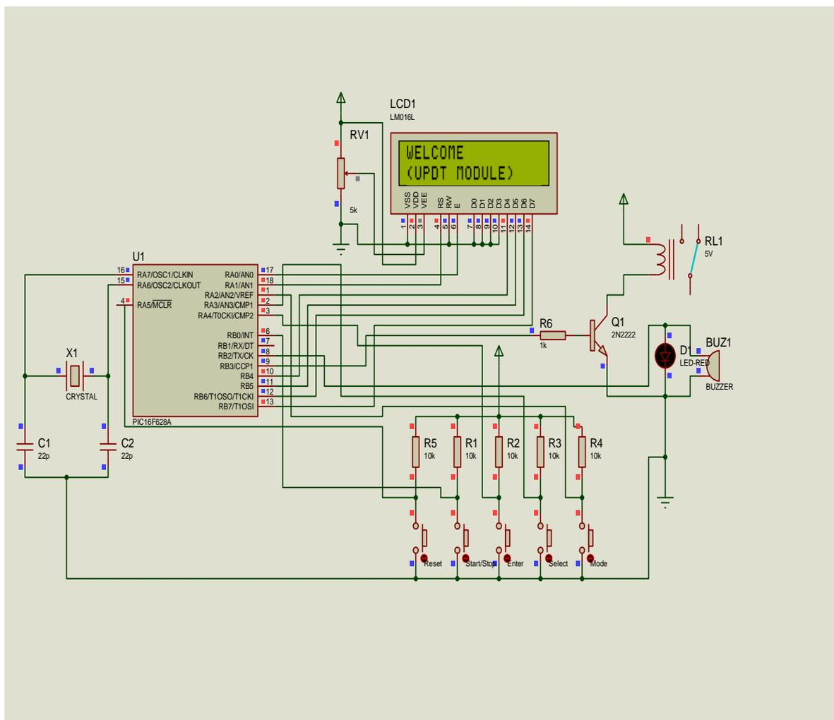
**Fig.4.** Simulated Circuit diagram of the module
