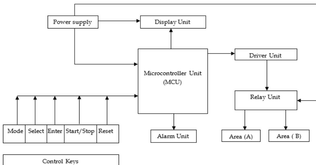
**Fig. 1.** The block diagram of the proposed UPDT switch
