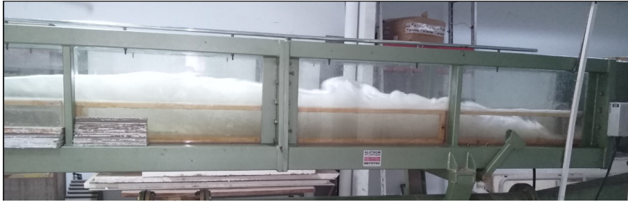
Fig.3. Hydraulic jump in a rectangular channel of a composite section with a rough minor bed
