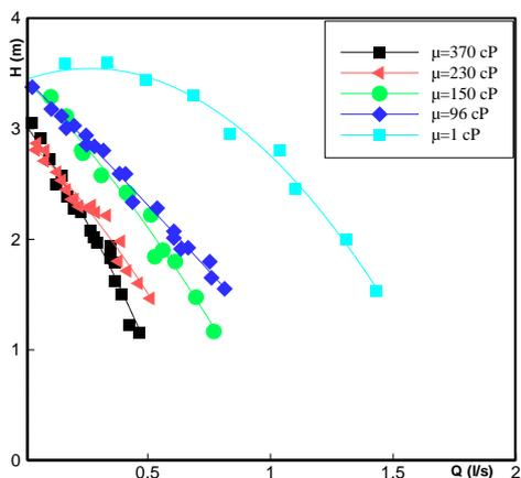
**Fig.15.** Head versus flow rate
