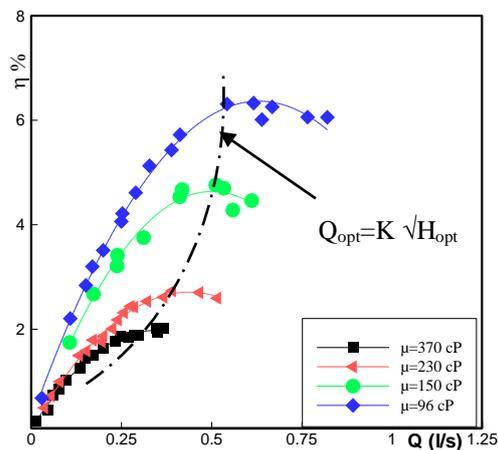
**Fig.17.** Efficiency versus flow rate
