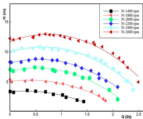
**Fig.8.** Head versus flow rate
