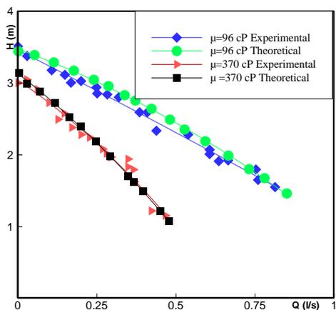
**Fig.13.** Head versus flow rate
