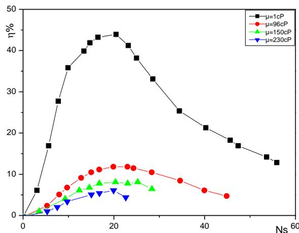
**Fig. 19.** Efficiency versus  $N_s$
