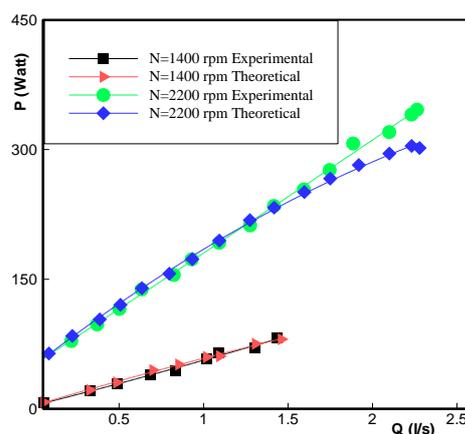
**Fig.7.** Power versus flow rate ( $\mu=10^{-3}$  Pa.s)
