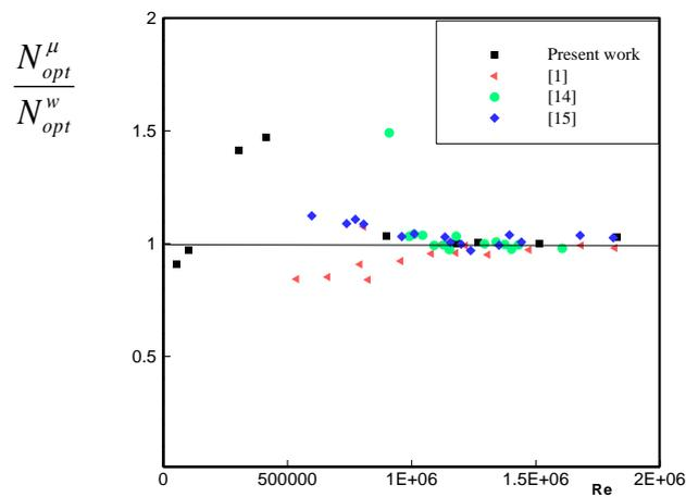
**Fig.20.** Ratio of the specific velocity as a function of  $Re$  at the points of best efficiency for viscous fluids and water
