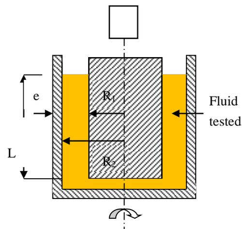
**Fig.3.** Couette viscometer
