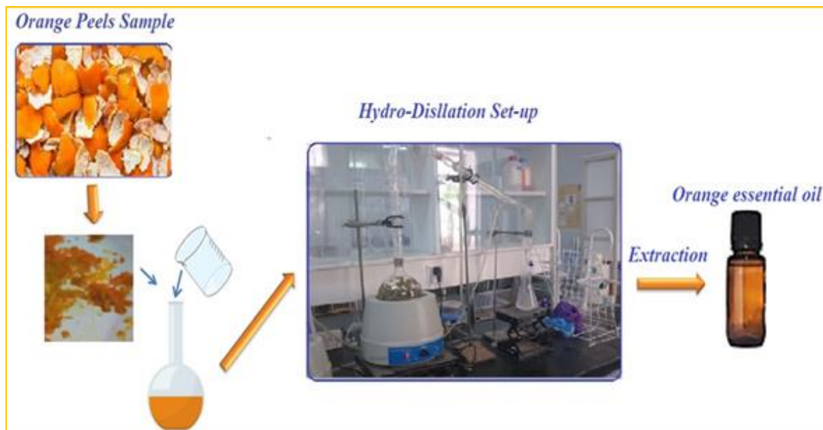
Fig.1. Extraction of orange essential oil by hydro-distillation
