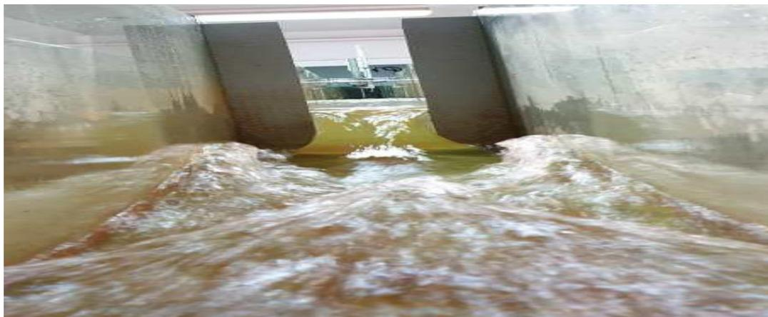
**Photograph 3.** Rectangular weir used to measure spill blades
