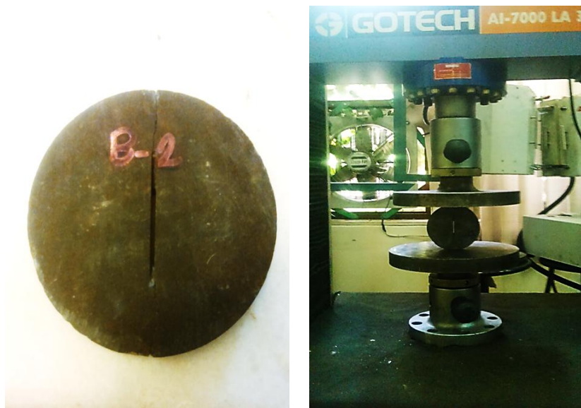
Fig.5. Fracture testing mechanism and sample after fracturing for CCNBD test
