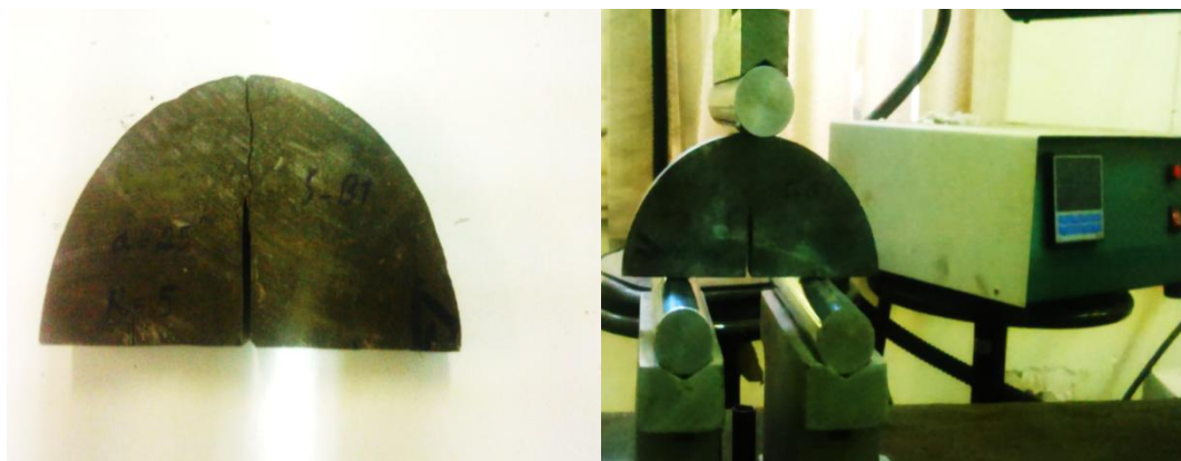
Fig.7. Fracture testing mechanism and sample after fracturing for SCB test.
