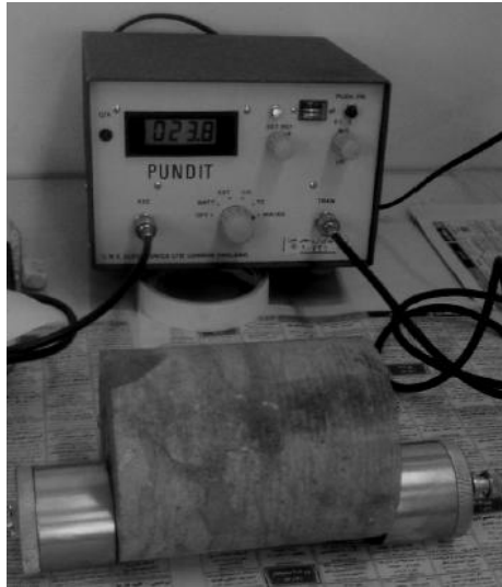
Fig.3. Ultrasonic tests of shear and compaction wave velocity per ASTM D-2845
