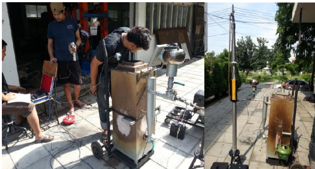
Fig.7. Updraft wood gasifier with gas flow meter experimental setup
