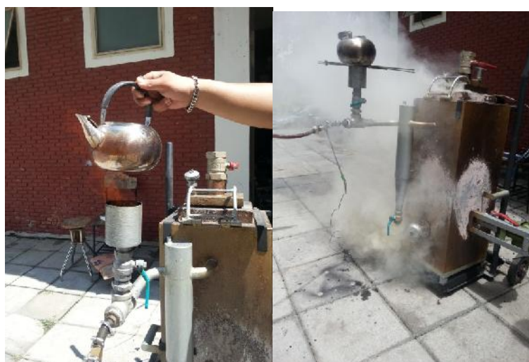
Fig.8. Water boiling by using Golden Shower tree biomass and charcoal as fuel
