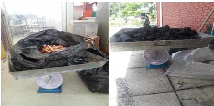
Fig.5. Weight measurement of Golden Shower tree biomass and charcoal
