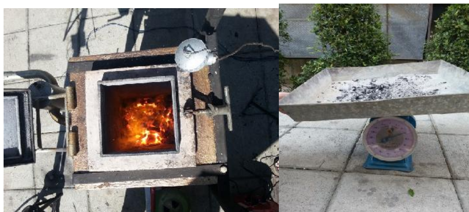
Fig.9. Gasifier combustion and ash weight measurement subsequently the test
