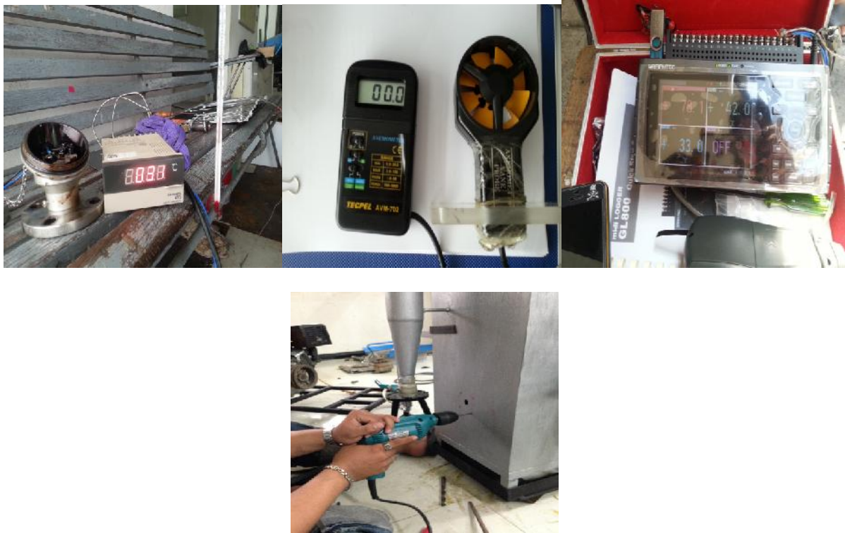
Fig.10. Measurement and instrumentation preparing for the experiment. (R type Thermocouple, glass thermometer, anemometer, data logger and hole drilling to insert thermocouple probe in the combustion chamber)
