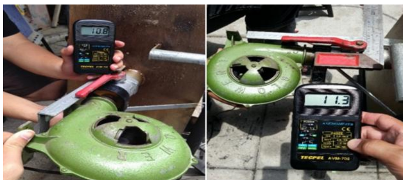
Fig.6. Air intake valve position, velocity measurement
